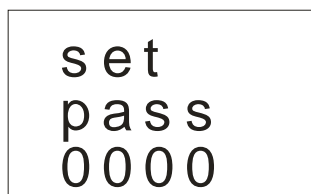
Figure 60. Password request to protect Set-up data
