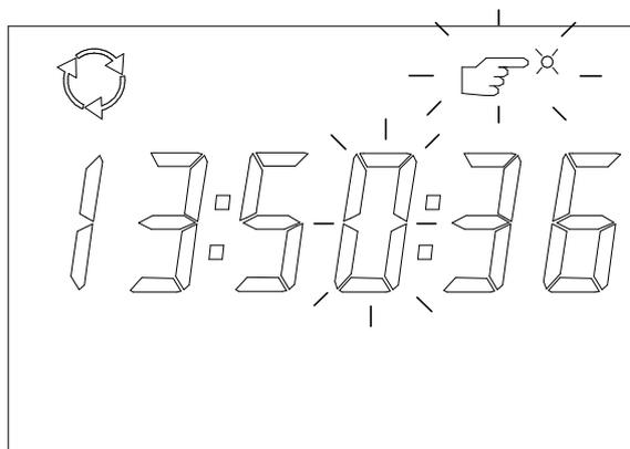
The second digits then starts flashing and is set to zero at every short press on the SCROLL button. The second digits are confirmed by pressing the SET button which completes the time set operation.
