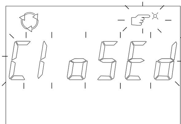
For every short press on the SCROLL button the state switches between "open" and "closed"
