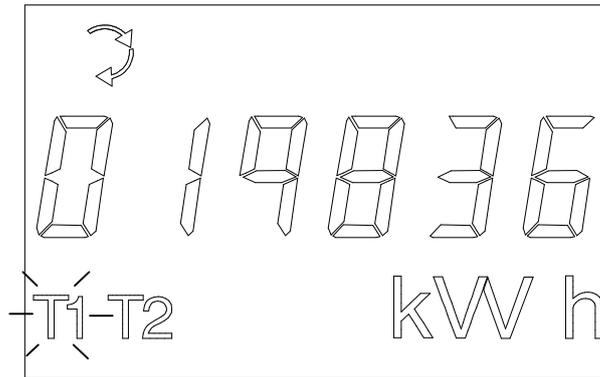
*Fig. 2-11 Normal Mode energy display*
