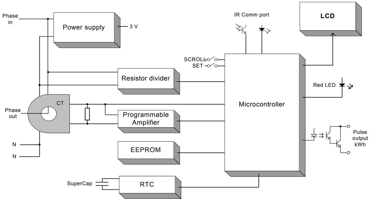
*Fig. 2-15 Electronics block diagram*
