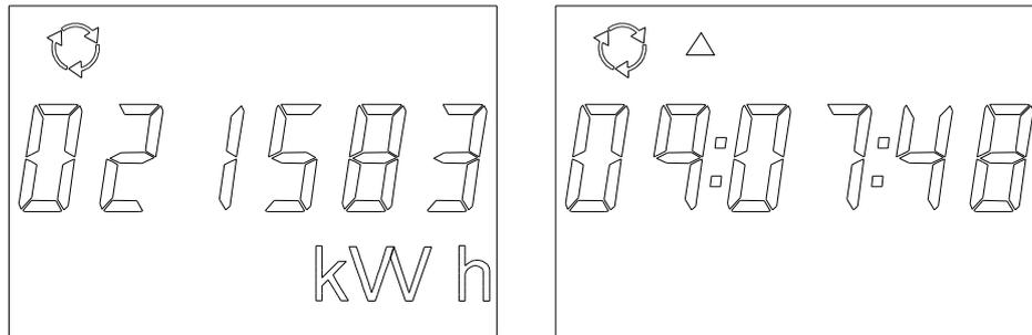
*Fig. 2-6 Display of active energy and time*
