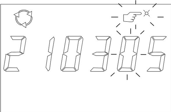
The year unit digit then starts flashing and is increased at every short press (possible values 0-9) on the SCROLL button. When the chosen value is confirmed by pressing the SET button the new date is set.
