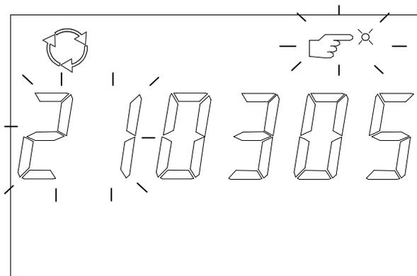
The day digits are increased by 1 for every short press (possible values 1-31) on the SCROLL button. The chosen value is confirmed by pressing the SET button.
