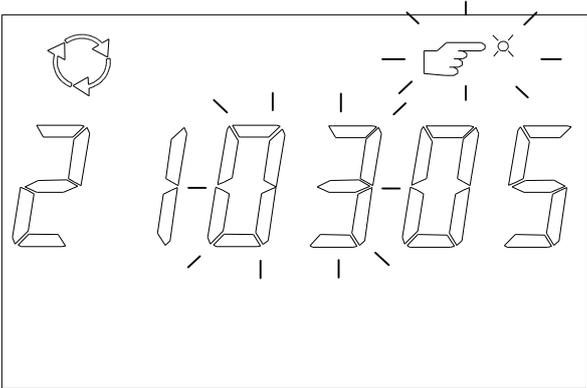
The year tens digit then starts flashing and is increased for every short press (possible values 0-9) on the SCROLL button. The chosen value is confirmed by pressing the SET button.
