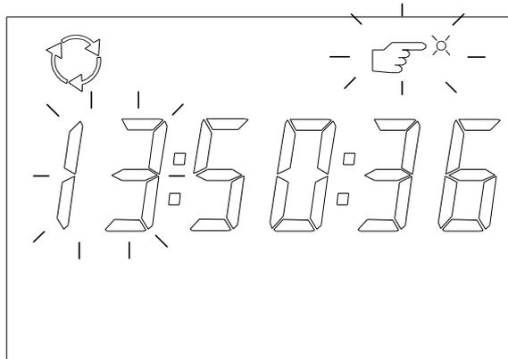
The hour digits are increased by 1 for every short press (possible values 0-23) on the SCROLL button. The chosen value is confirmed by pressing the SET button.
