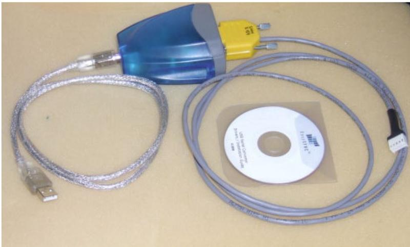
A driver installation CD is provided with the programming adapter.
