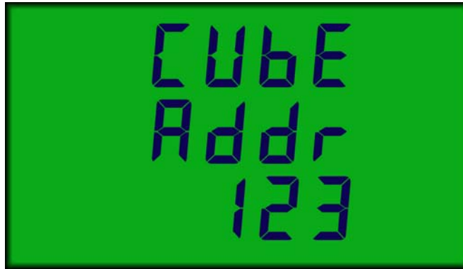
Figure 3-2 Setting The Modbus Address
