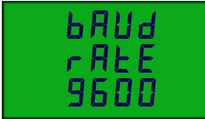
Figure 3-1 Setting The Baud Rate
