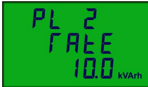
Figure 4.3 Setting The Pulse Output #2 Rate
