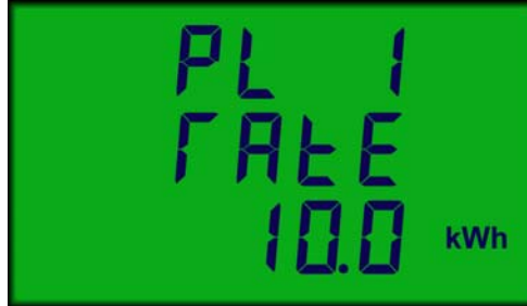
Figure 4.2 Setting The Pulse Output #1 Rate
