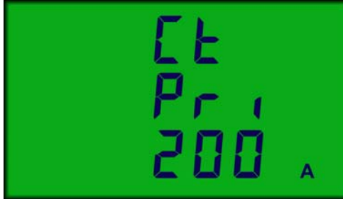
Figure 4.1 Setting The CT Primary Constant
