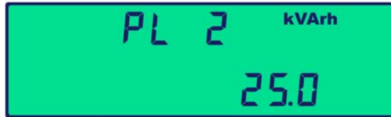
Figure 4.3 Setting The Pulse Output #1 Rate
