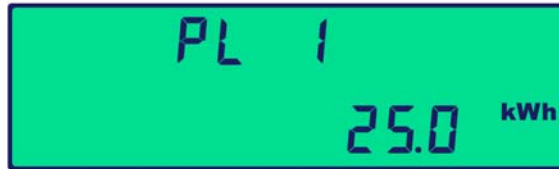
Figure 4.2 Setting The Pulse Output #1 Rate
