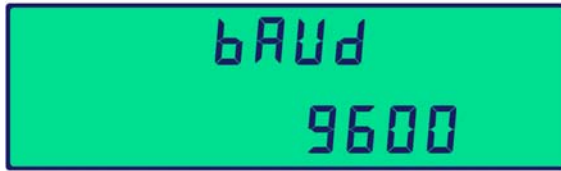
Figure 4.7 Setting the Baud Rate
