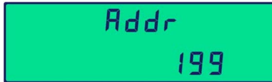
Figure 4.6 Setting the Modbus Address
