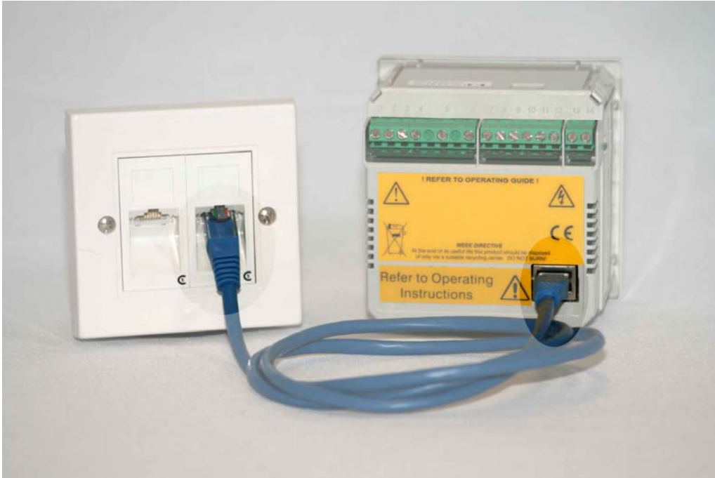
Figure 4. Meter Network Connection
