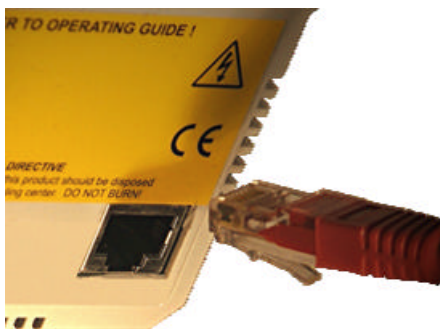
Standard RJ45 network connector on rear of the Meter
