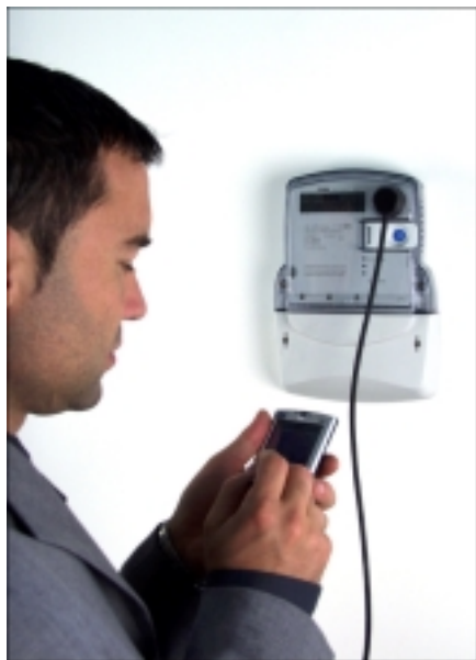
Fig. 6 – Data downloading by means of a Palm top PC is shown
