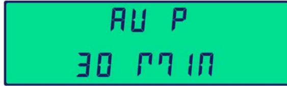
Figure 4.5 Setting kW Rolling Demand Period
