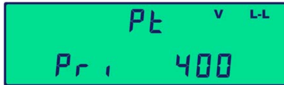
Figure 4.1 Setting The PT Primary Constant
