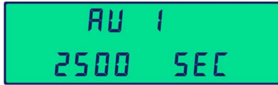
Figure 4.4 Setting Ampere/Voltage Demand Period
