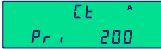
Figure 4.1 Setting The CT Primary Constant
