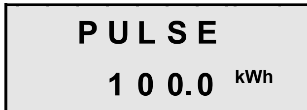
Figure 4.3 Setting The Pulse Output Rate
