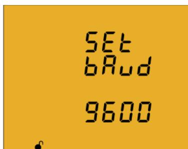
The transmission speed of BACnet communications is programmed on this screen.
