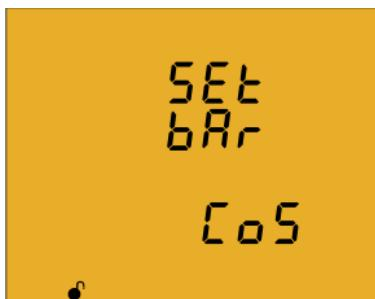
This screen is used to select the Cos φ - PF bar viewing option.
