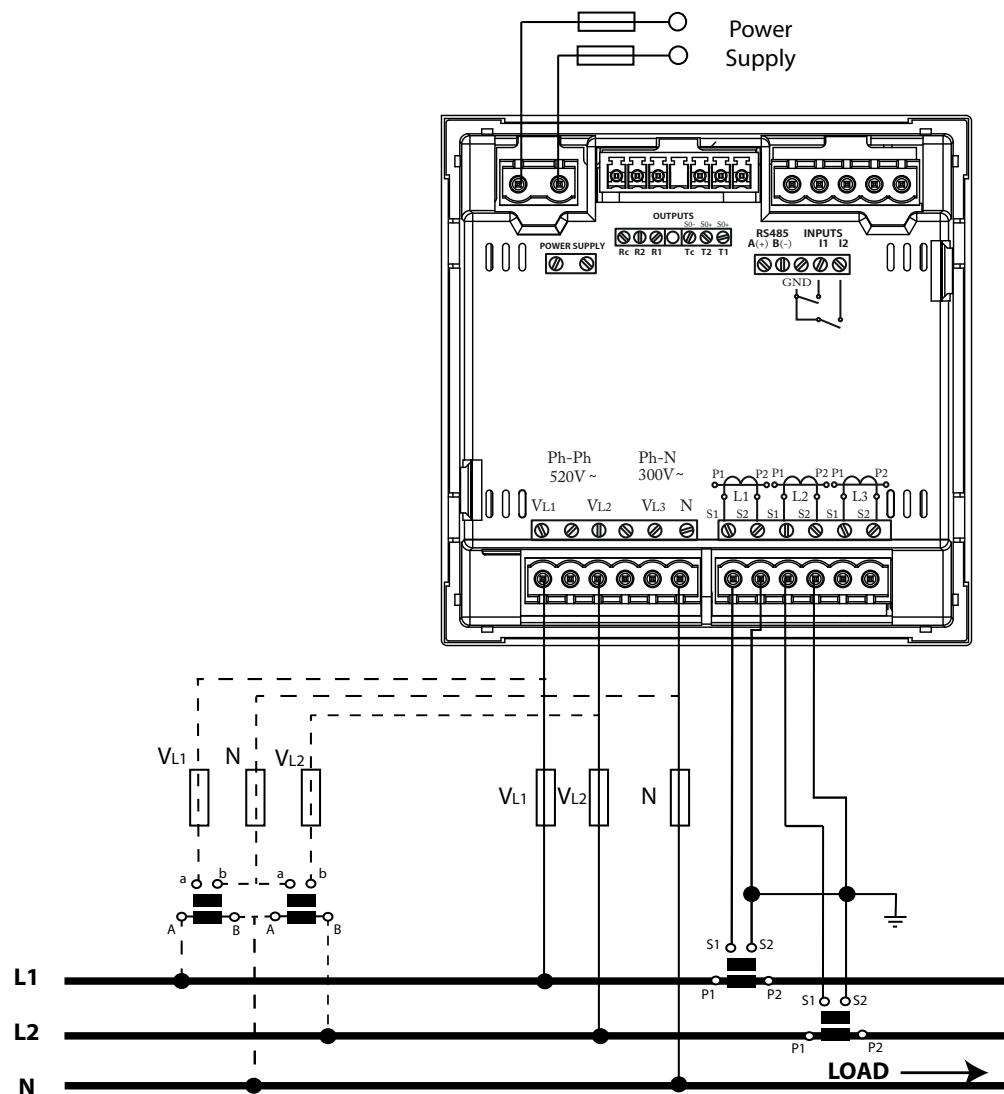
Figure 9: Measuring Two-Phase Networks with a 3-wire connection, CVM-C10-ITF, CVM-C10-MC and CVM-C10-mV models.
