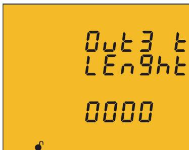
The width of the pulse is selected on this screen in ms.
