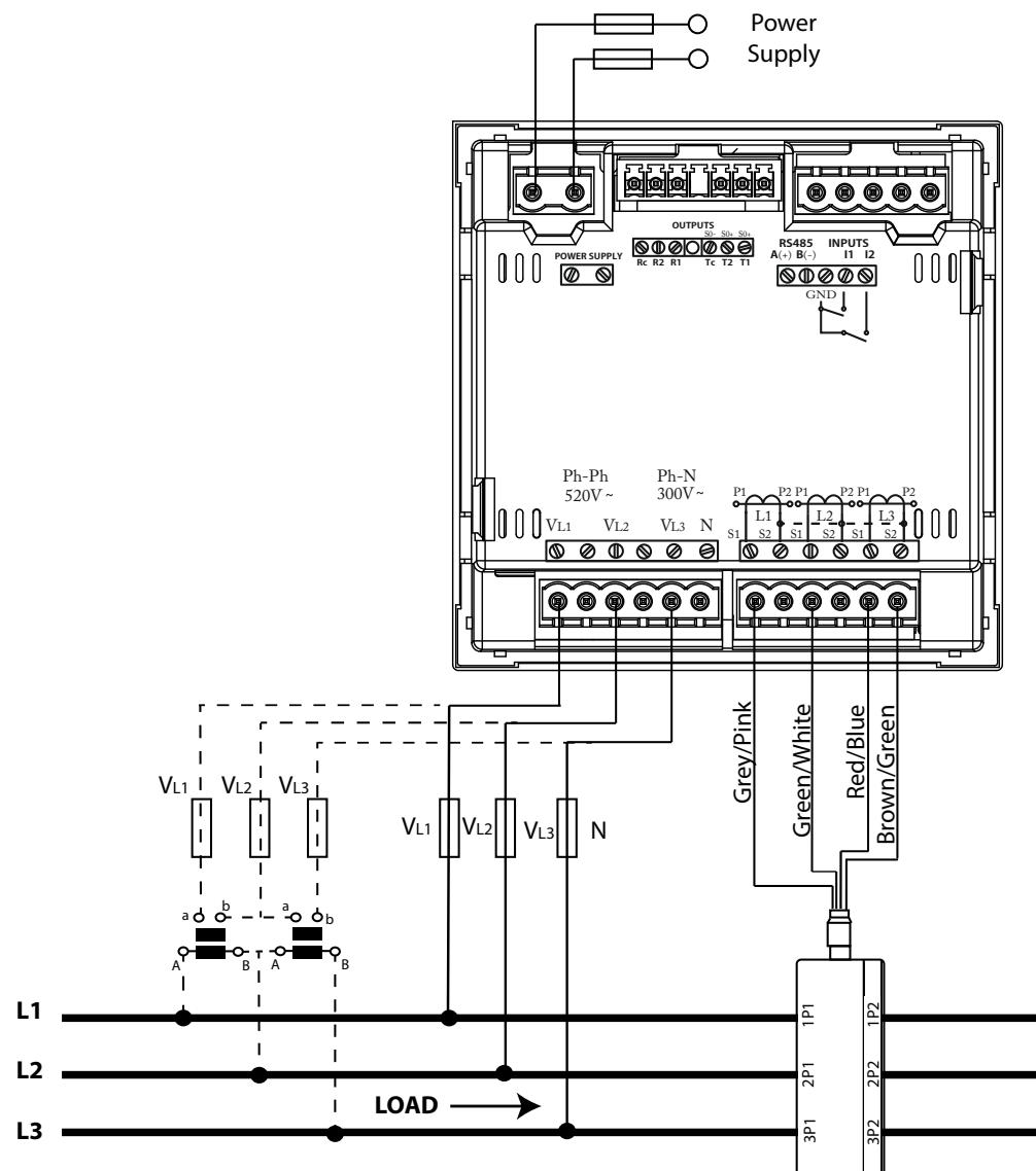
Figure 7: Three-Phase measuring with a 3-wire connection, CVM-C10-MC model.
