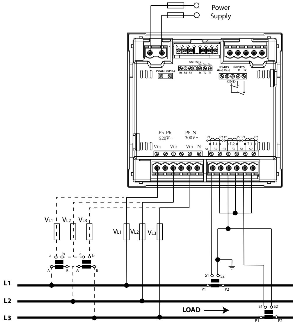
**Figure 8:** Three-Phase measuring with a 3-wire connection and transformers with an ARON connection, CVM-C10-ITF, CVM-C10-MC and CVM-C10-mV models.
