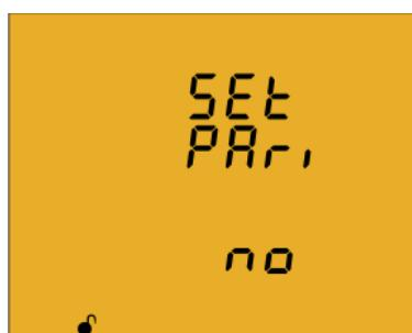
The type of parity of Modbus communications is selected on this screen.
