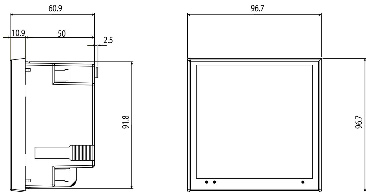
Figure 26: Dimensions of the CVM-C10.
