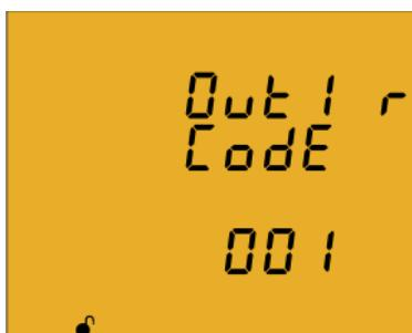
The variable code is selected on this screen, depending on **Table 12**, which will control alarm relay 1.
