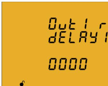
The alarm connection delay is programmed on this screen in seconds.
