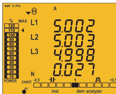
Figure 21: Analyzer profile screen displaying the maximum demand values.
