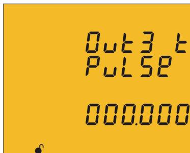
Press key for 3 seconds to edit the kilowatts per pulse selection. The **prog** icon will be displayed on the bottom of the screen.
