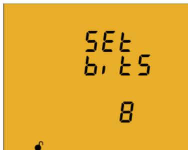
The number of data bits of Modbus communications are programmed on this screen.
