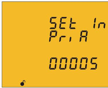
The neutral current transformer primary is programmed on this screen.
