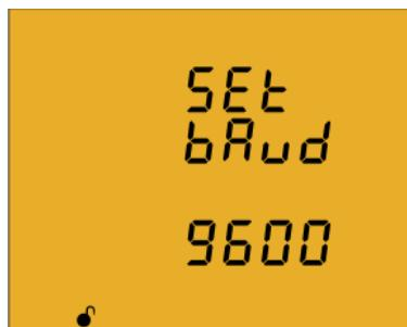
The transmission speed of modbus communications is programmed on this screen.
