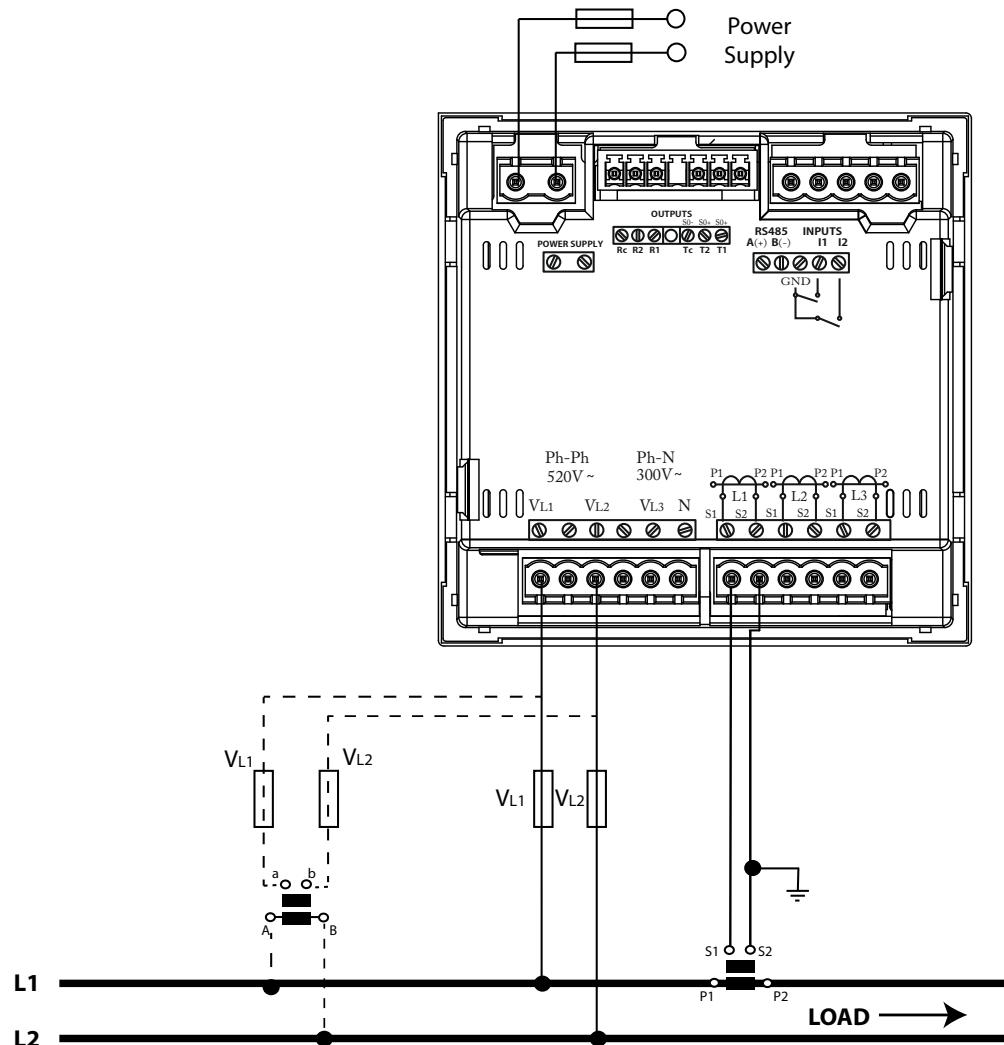
Figure 11: Measuring Single-Phase Networks, phase to phase, with a 2-wire connection, CVM-C10-ITF, CVM-C10-MC and CVM-C10-mV models.
