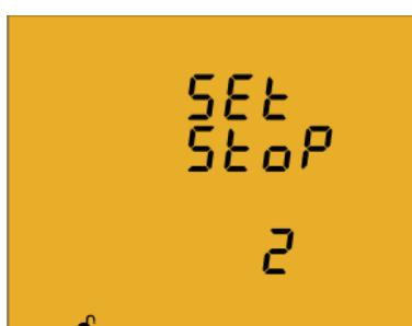
The number of Stop bits of Modbus communications are programmed on this screen.
