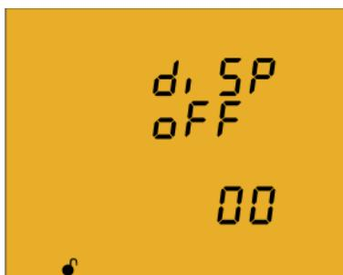
The time that the Backlight will stay lit (in seconds) is programmed on this screen after the last keystroke on the unit .
