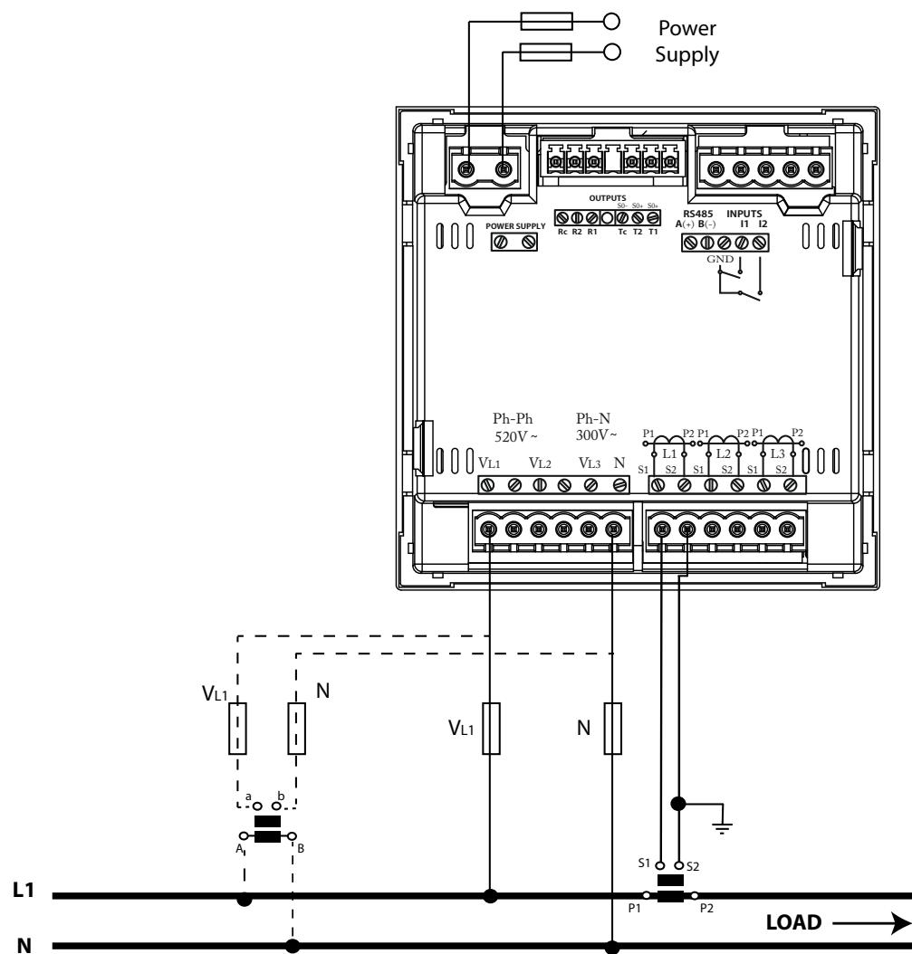
**Figure 12: Measuring Single-Phase Networks, phase to neutral, with a 2-wire connection, CVM-C10-ITF, CVM-C10-MC and CVM-C10-mV models.**
