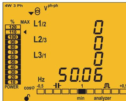
Figure 20: Analyzer profile screen displaying the minimum values.
