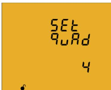
Press key **≡** for 3 seconds to edit the number of quadrants. The **prog** icon will be displayed on the bottom of the screen.
