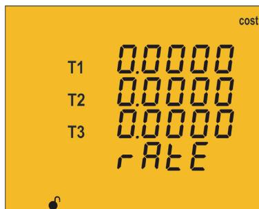
The cost per kWh of electricity of the three tariffs of the unit is calculated on this screen.
