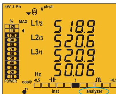
Figure 18: CVM-C10 screen with the analyzer profile.
