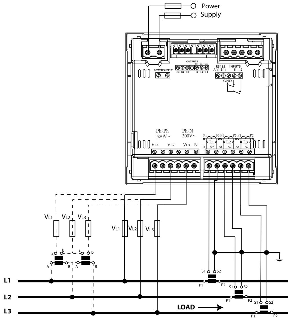
Figure 6: Three-Phase measuring with a 3-wire connection, CVM-C10-ITF and CVM-C10-mV model.
