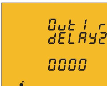
The alarm disconnection delay is programmed on this screen in seconds.
