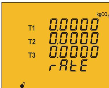
The carbon emissions ratio is the amount of emissions released into the atmosphere to produce a unit of electricity (1 kWh). The ratio for the European mix is approximately 0.65 kgCO<sub>2</sub> per kWh.
