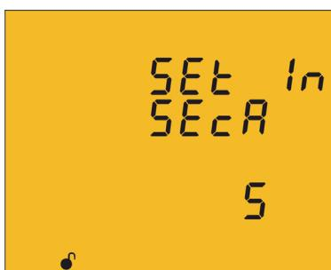
The neutral current transformer secondary is programmed on this screen.
