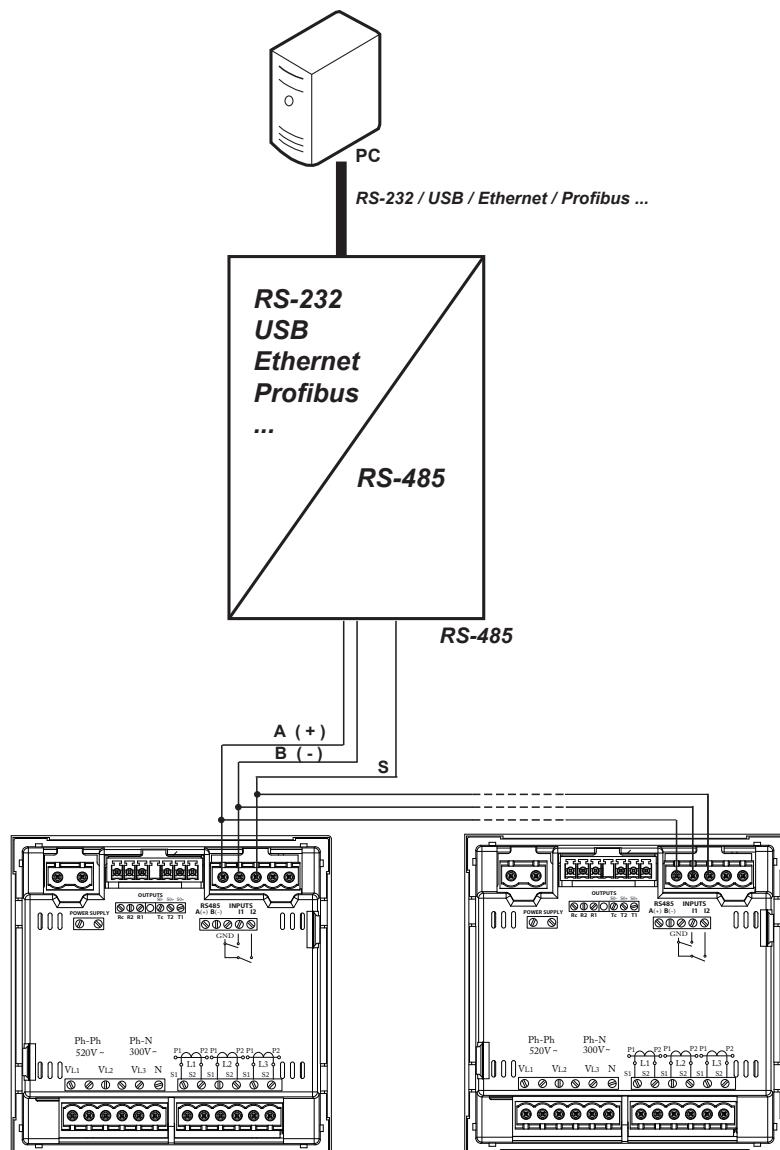
Figure 25: RS-485 Connection diagram.
