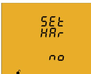
This screen is used to select whether harmonics are displayed or not.
