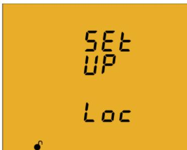
This screen is for protecting the data configured in the programming menu.
