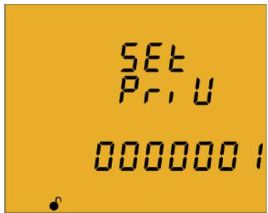
On this screen the voltage transformer primary is programmed.
