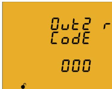
The values for alarm relay 2 are programmed on this screen.
