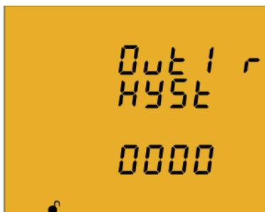
The hysteresis value, i.e., difference between the alarm connection and disconnection value, in %, is programmed on this screen.
