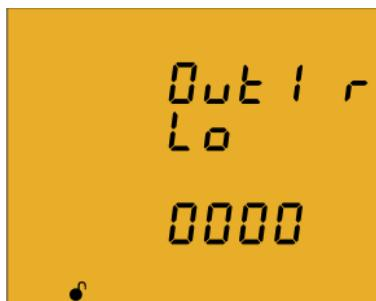
The **minimum value**: the alarm is activated below this value. Press key **≡** for 3 seconds to edit the minimum value selection. The **prog** icon will be displayed on the bottom of the screen. To enter or modify the value, press the **≡** key repeatedly, increasing the value of the flashing digit.
