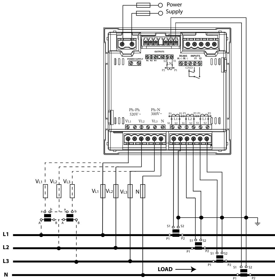
Figure 4: Three-Phase Measuring with a 4-wire connection, CVM-C10-ITF-IN model.
