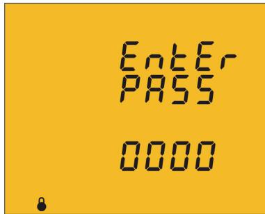
Enter the password in this screen to modify the programming parameters.
