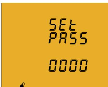
On this screen you enter the password for locking and unlocking the programming.
