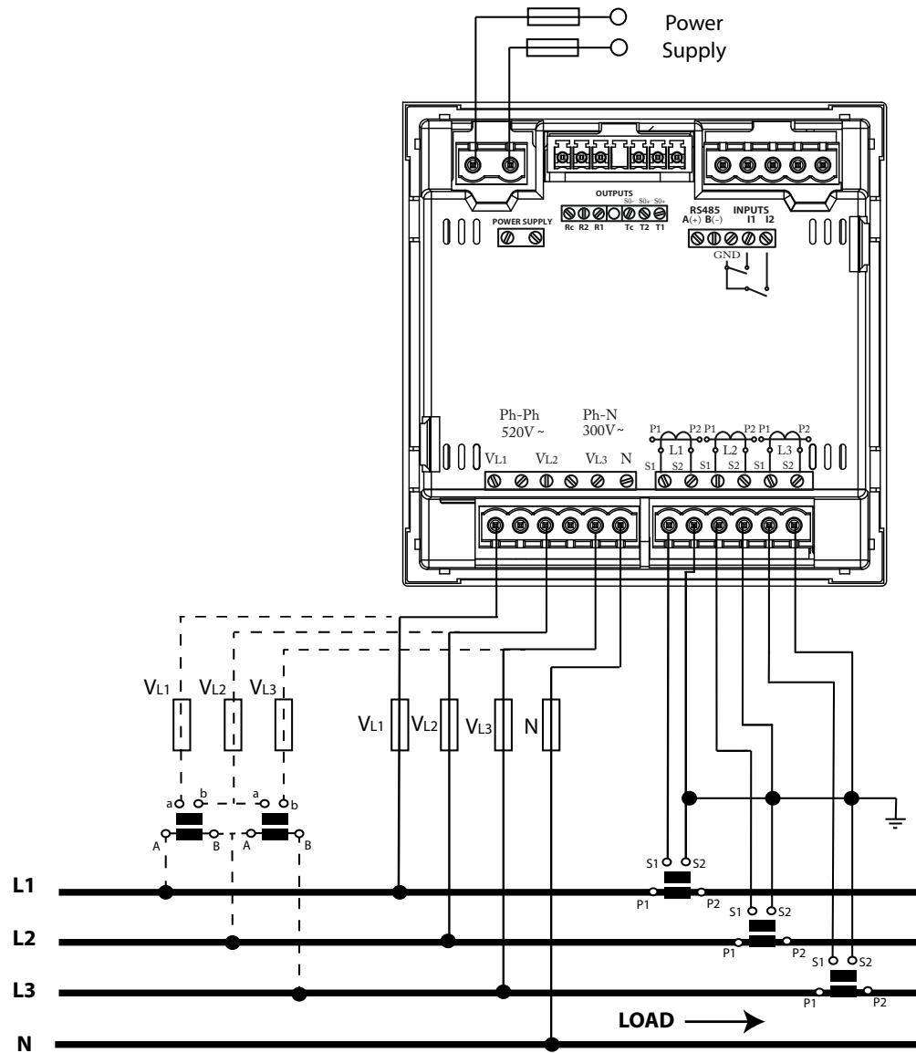
Figure 3: Three-Phase measuring with a 4-wire connection, CVM-C10-ITF and CVM-C10-mV model.
