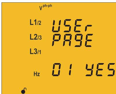
This screen displays the first screen of the **analyzer** profile, **Phase-phase Voltage** and the **user** profile viewing option can be selected.
