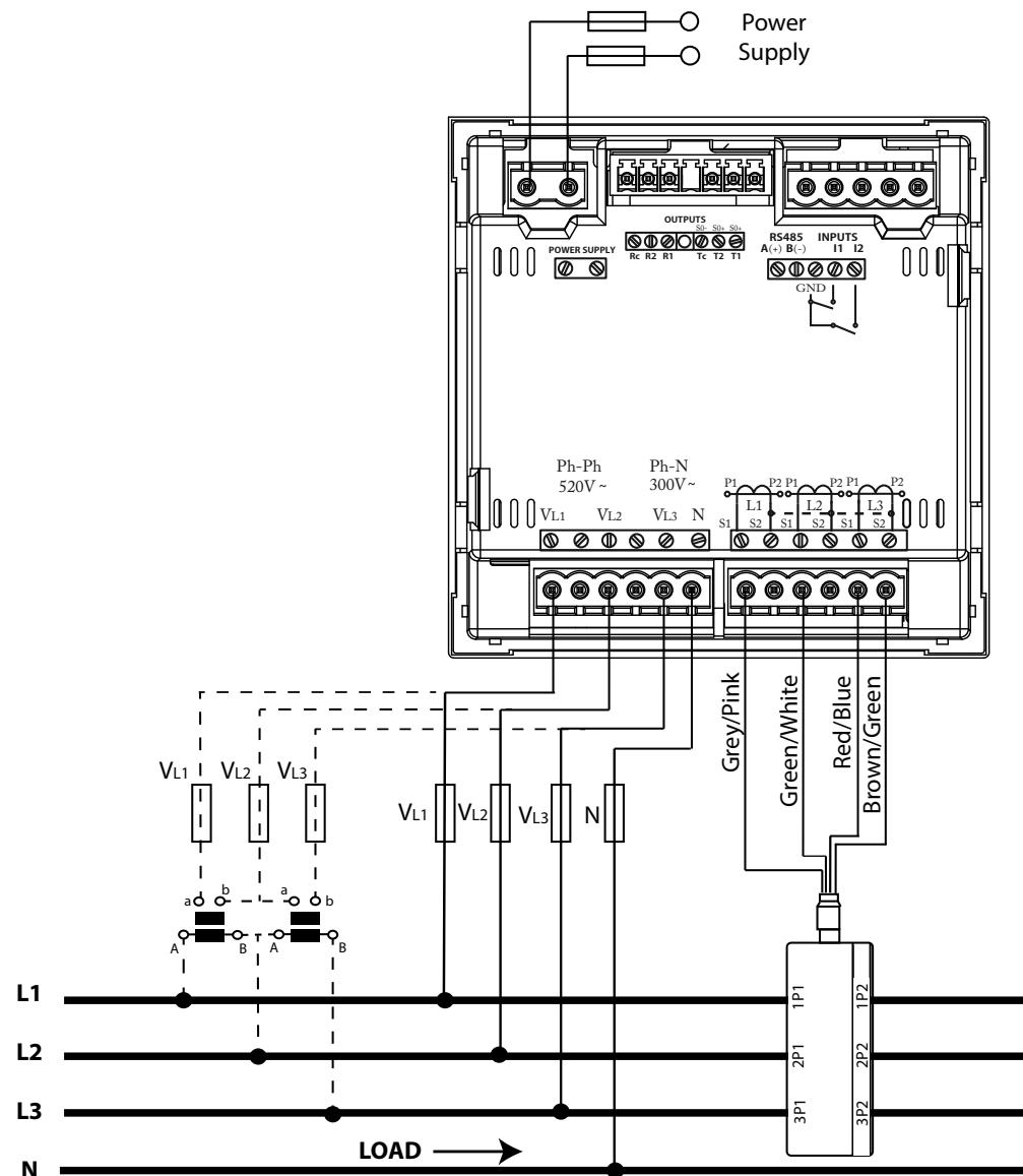
Figure 5: Three-Phase measuring with a 4-wire connection, CVM-C10-MC model.
