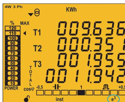
Figure 22: CVM-C10 screen with the **e<sup>3</sup>** profile.
