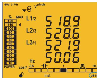
Figure 23: Screen of the CVM-C10 with the user profile.
