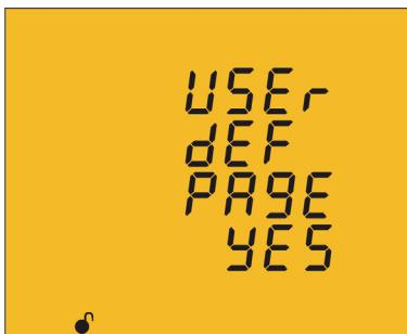
This screen is used to select whether the unit's display screens are defined by the user or not.
