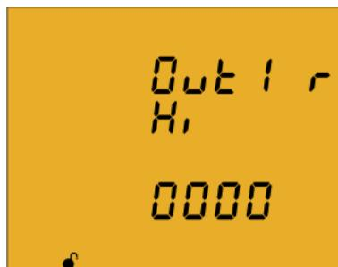
The **maximum value**: the alarm is activated when this value is exceeded.
