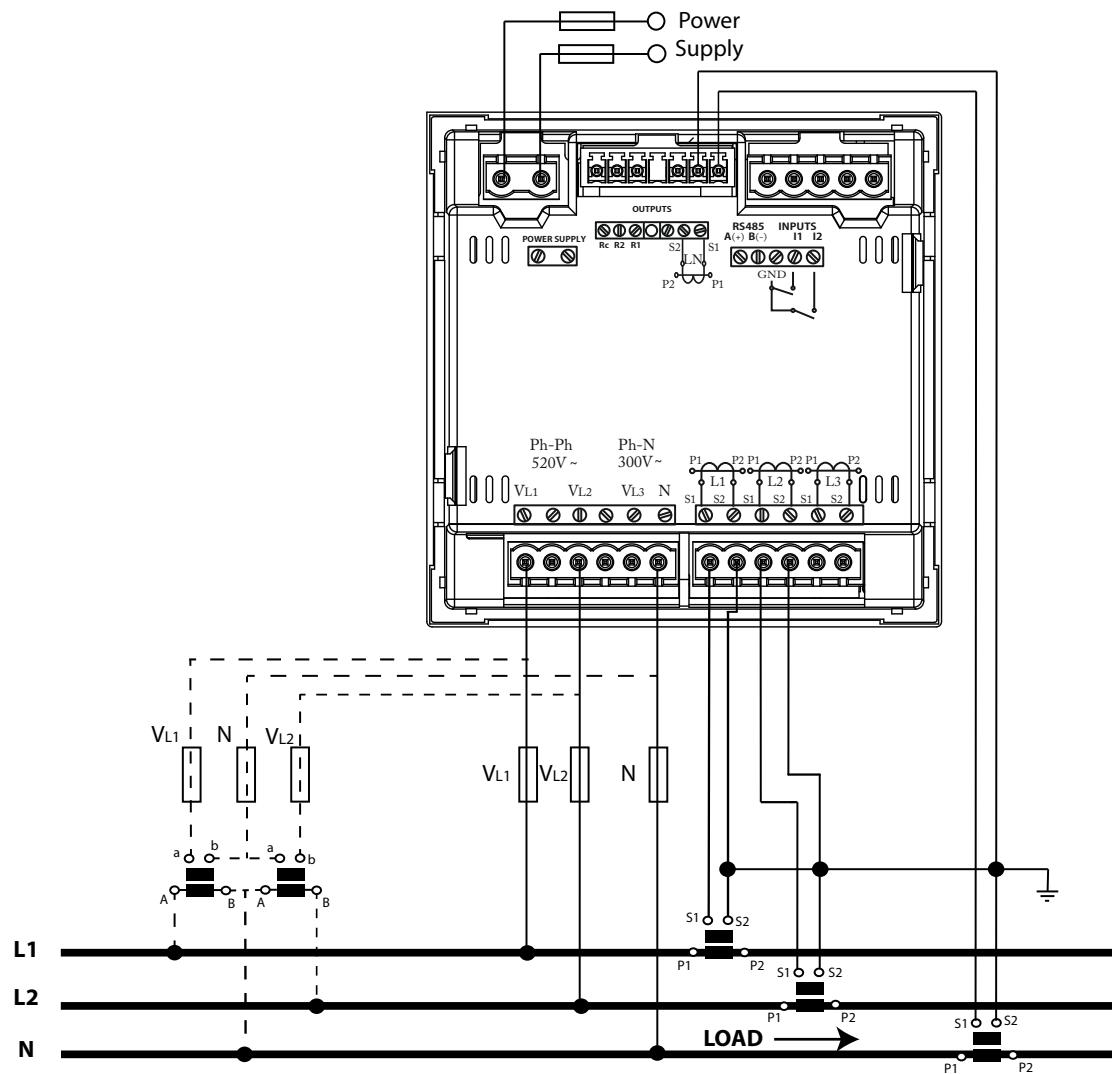
Figure 10: Measuring Two-Phase Networks with a 3-wire connection, CVM-C10-ITF-IN model.
