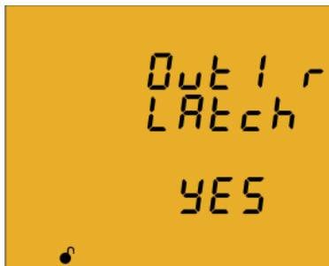
The interlocking is selected on this screen, i.e., if the alarm is interlocked after it has been tripped, even when the condition that triggered it has disappeared.
