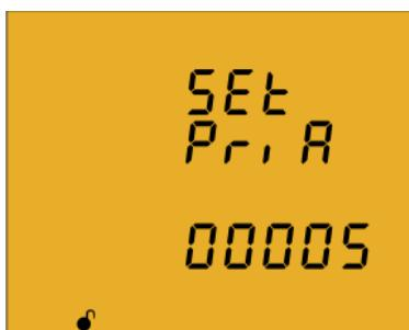
The current transformer primary is programmed on this screen. Press key **≡** for 3 seconds to edit the transformer primary value. The **prog** icon will be displayed on the bottom of the screen.
