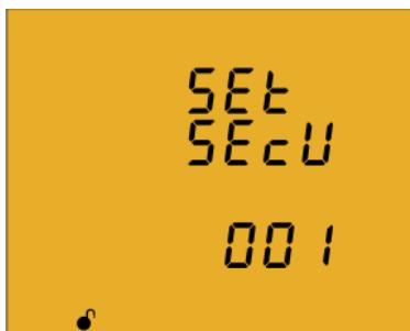
On this screen the voltage transformer secondary is programmed. Press key **≡** for 3 seconds to edit the transformer secondary value. The **prog** icon will be displayed on the bottom of the screen.
