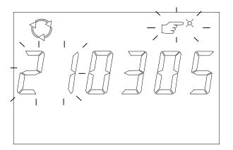
The day digits are increased by 1 for every short press (possible values 1-31) on the SCROLL button. The chosen value is confirmed by pressing the SET button.
