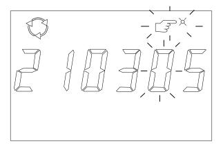
The year unit digit then starts flashing and is increased at every short press (possible values 0-9) on the SCROLL button. When the chosen value is confirmed by pressing the SET button the new date is set.
