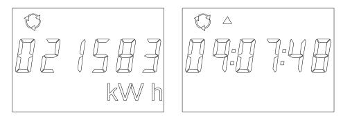
Fig. 2-6 Display of active energy and time
