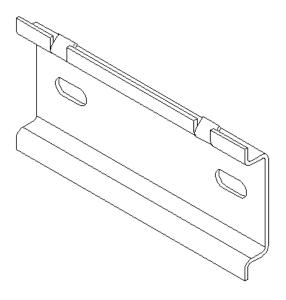
Fig. 4-1 DIN-rail used for wall mounting
