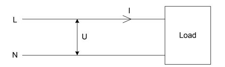
Fig. 5-1 Single phase measurement.
