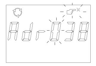
The first digit is increased by 1 for every short press on the SCROLL button. Possible values for the first digit are 0-2. The chosen value is confirmed by pressing the SET button. The same procedure is then done for the 2 other digits (possible values for these two digits are 0-9). When the last digit is confirmed the meter will start to use the new address. It is only possible to select valid addresses (1 to 250).
