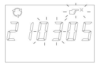
The year tens digit then starts flashing and is increased for every short press (possible values 0-9) on the SCROLL button. The chosen value is confirmed by pressing the SET button.
