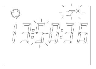
The minute unit digit then starts flashing and is increased for every short press (possible values 0-9) on the SCROLL button. The chosen value is confirmed by pressing the SET button.
