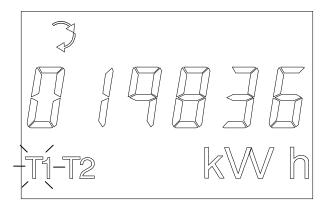
Fig. 2-11 Normal Mode energy display
