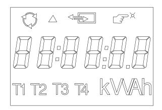
Fig. 2-12 LCD test
