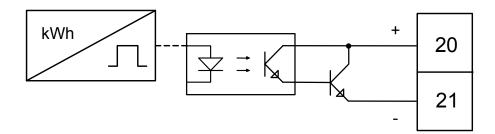
Fig. 2-14 Pulse output equivalent schematic diagram
