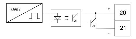
Fig. 2-11 Pulse output equivalent schematic diagram
