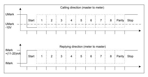
Fig. 6-1 Transmission of a Character in Calling and Replying Direction
