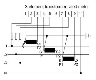
Fig. 4-2 Wiring diagram for transformer connected meter
