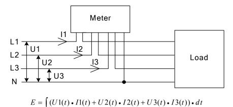
Fig. 5-1 3-element measurement
