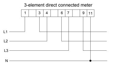
Fig. 4-1 Wiring diagram for direct connected meter
