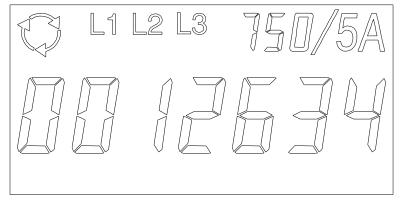
Fig. 2-10 Display of current transformer ratio 750/5
