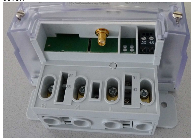
Fig. 30: SMA connector under the meter cover
