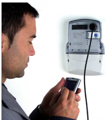
Fig. 28: Meter readout via an IR optical interface
