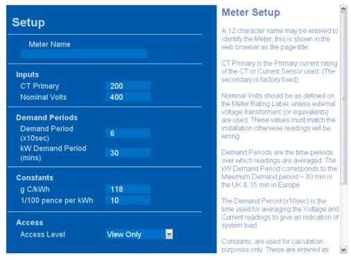
At the bottom of the screen the *Access* section contains a drop-down control that sets the level of control that the user has over the settings.
