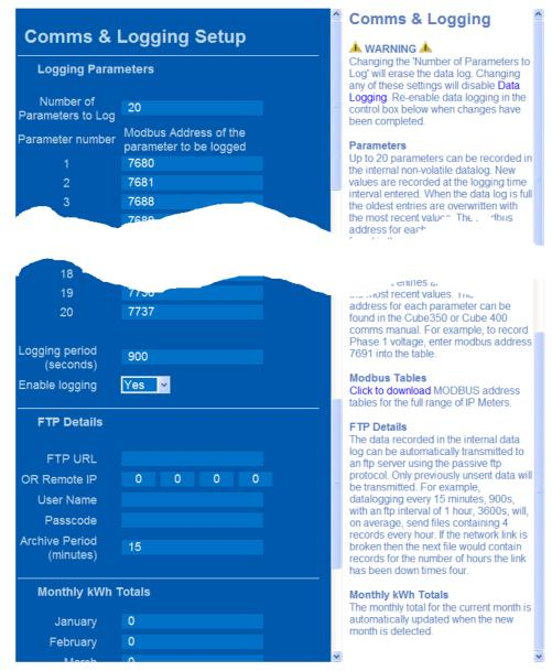
The first text box in the *Logging Parameters* section sets the number of parameter registers that are to be logged. Up to 20 registers can be logged. (Note that some parameters - such as the energies - are split into high and low portions and take up two registers in the list.) The parameters registers are entered into the table as MODBUS® addresses. For MODBUS® addresses see appendix A. A full list of MODBUS® addresses is also available for download from the Help page.
