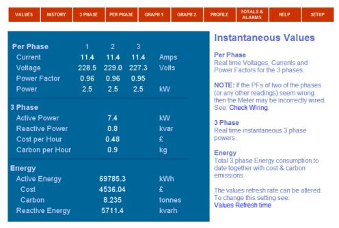
The Per Phase section displays individual values for each of the three phases.
