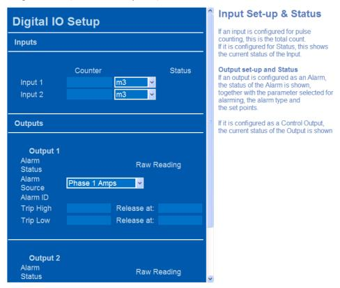
The *Inputs* section of this page allows the inputs to be configured.
