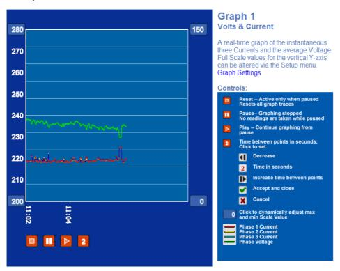
The graph starts plotting as soon as the page is loaded. Hovering the mouse over any point on a trace opens a small window displaying the actual data at that point. Clicking the pause button ( ) freezes the display; while frozen click the reset button ( ) to clear the display or the play button ( ) to resume plotting. The time interval button ( ) shows the interval between points in seconds, click on this button to change the interval.
