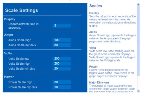
The *Display* text box sets the refresh time for displays of instantaneous values; this is the same as the time between points for the two graphs. Values between 1 and 60 seconds are allowed.
