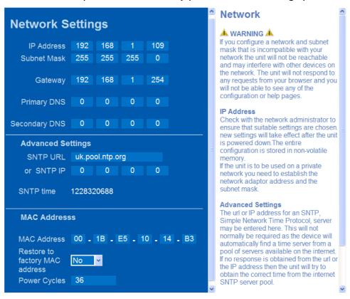
The meter is supplied with a default IP address of 192.168.1.127 and a subnet mask of 255.255.255.0. The DNS server addresses are only required if the meter is used for automatic remote data-logging.
