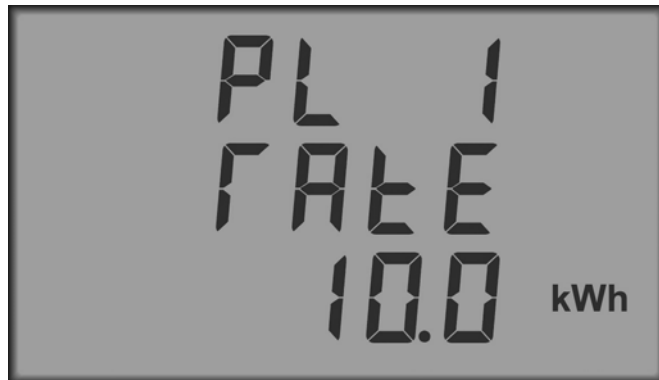
Figure 4-3 Setting The Pulse Output #1 Rate
