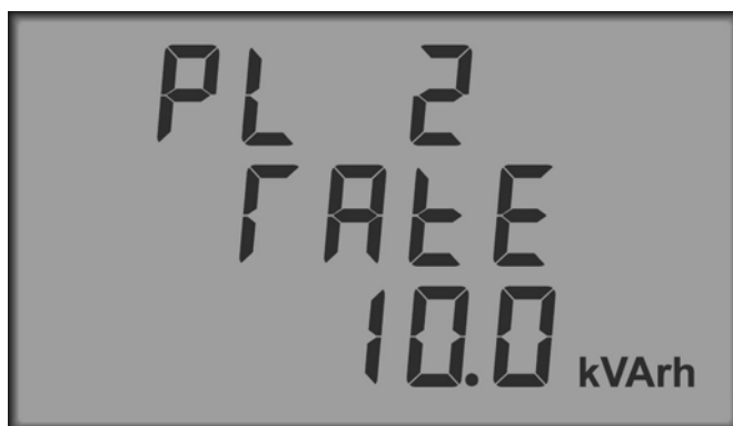
Figure 4-4 Setting The Pulse Output #2 Rate
