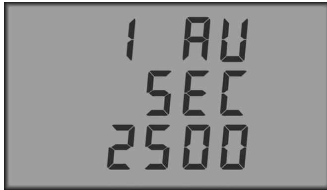
Figure 4-5 Setting Ampere/Voltage Demand Period
