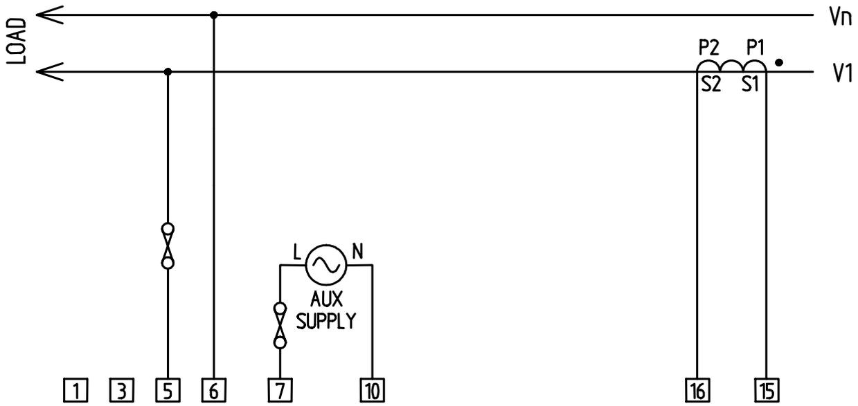
Figure 3-2 Single Phase Connection
