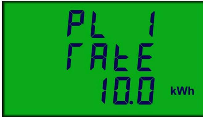
Figure 4-3 Setting The Pulse Output #1 Rate
