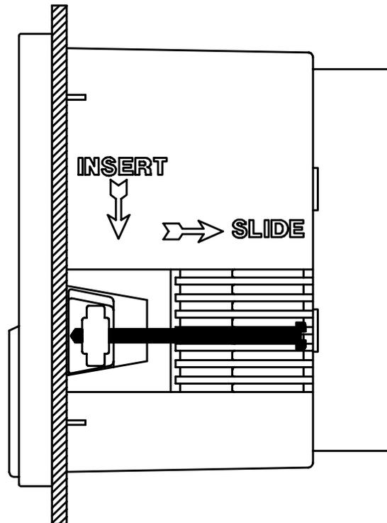
Figure 3-1 Fitting The Meter in a Panel
