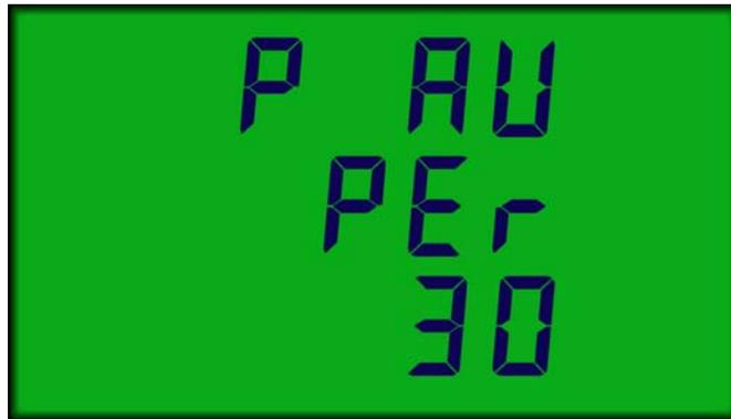
Figure 4-6 Setting Watts Rolling Demand Period
