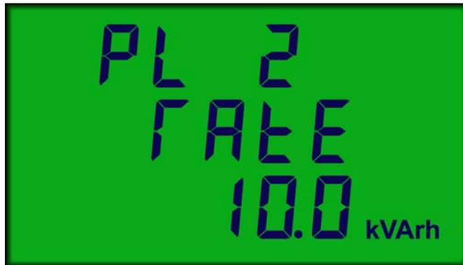
Figure 4-4 Setting The Pulse Output #2 Rate
