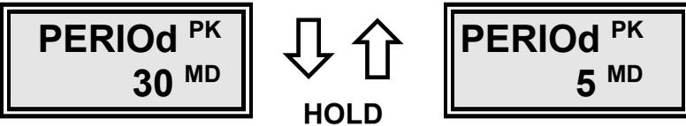
The new value is stored automatically in non-volatile memory and is secure in the event of power failure.
