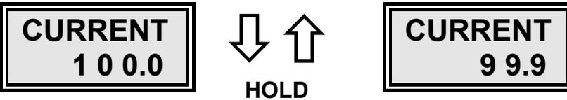
The new value is stored automatically in non-volatile memory and is secure in the event of power failure.
