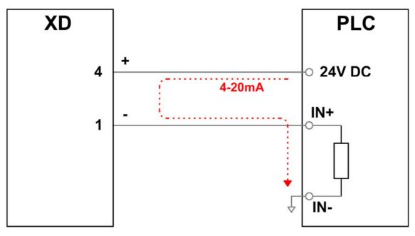
8. Typical 4-20mA Connection Loop Powered
