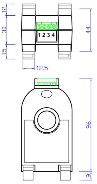
5. Dimensioned Drawing (Including Rail MountClips)
