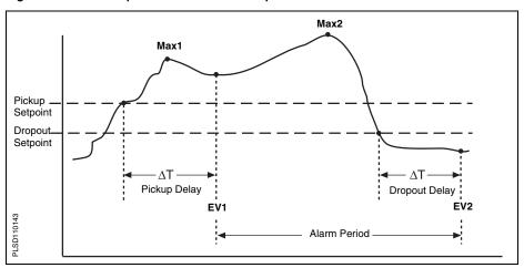
Figure 6-2: How the power meter handles setpoint-driven alarms
