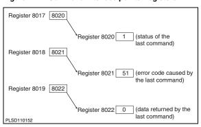
Figure B-1: Command interface pointer registers
