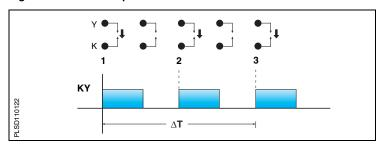
In Figure 5–3, the transitions are marked as 1 and 2. Each transition represents the time when the relay contact closes. Each time the relay transitions, the receiver counts a pulse. The power meter can deliver up to 12 pulses per second in a 2-wire application.
