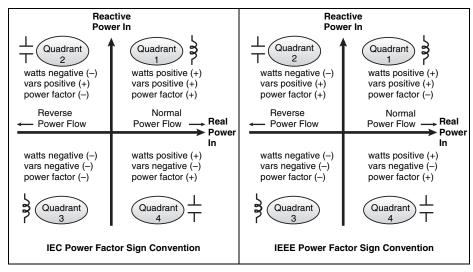
Figure 4-3: Power Factor Display Example
