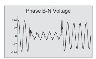
Figure 10–2: Waveform showing voltage sag caused by a remote fault and lasted five cycles
