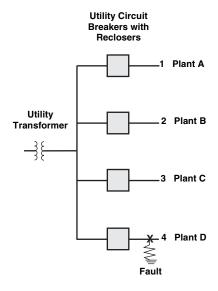
A fault near plant D, cleared by the utility circuit breaker, can still affect plants A, B, and C, resulting in a voltage sag.
