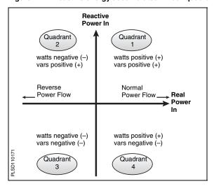
Figure 4-7: Reactive energy accumulates in four quadrants
