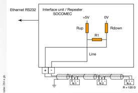
Diagram of a bus connection with SOCOMEC interface units with integrated biasing
